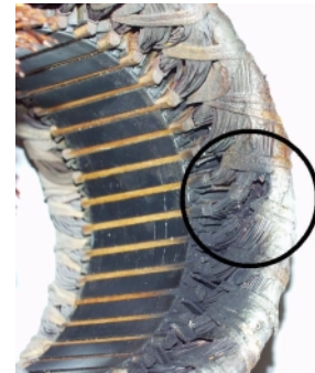
Damage from winding turn to turn fault
